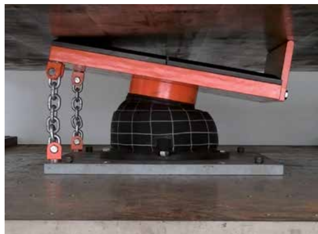
SPC Fender angular compression testing with restrain chains
