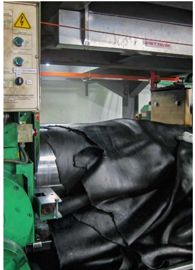
Finalized compound on rolling mill
