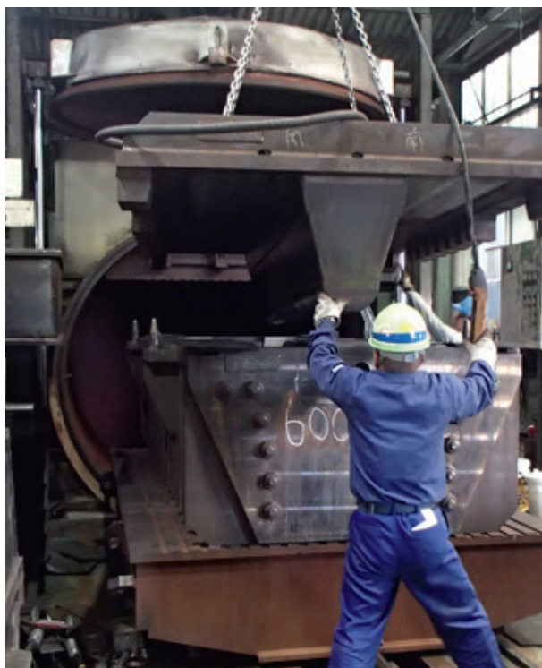
Closing mold with counterpart prior to curing
