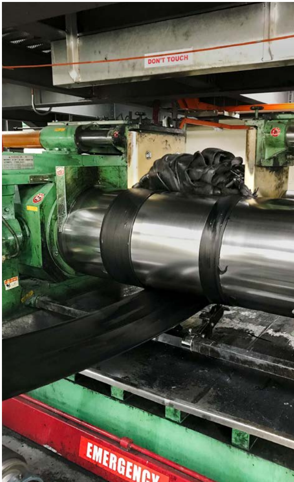
Masterbatch on rolling mill
