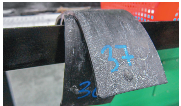
Test specimen from final compound for material testing
