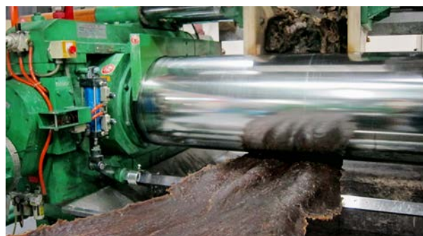
Masticated rubber on rolling mill
