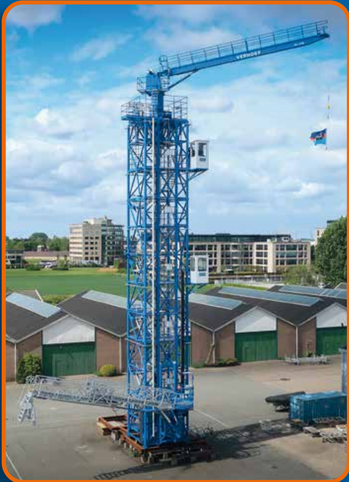
Tower with lift platforms, telescopic gangway and stores crane. Gothenburg - Sweden
