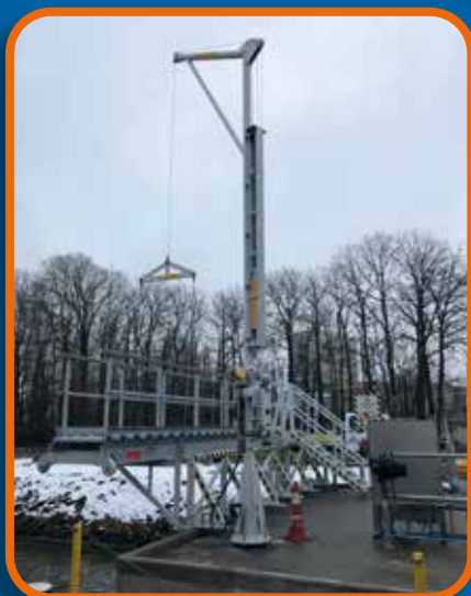
Riding access ladder with hoisting davit. Ghent - Belgium
