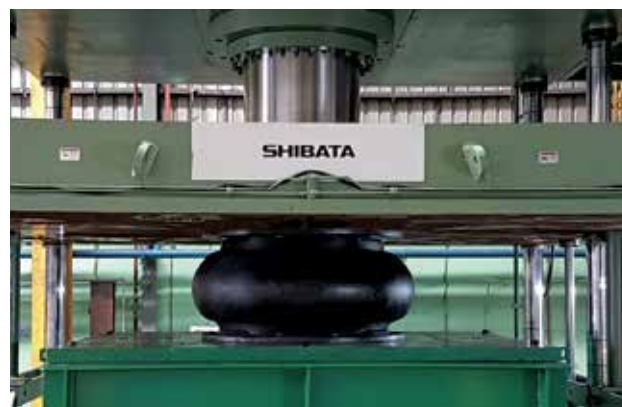
Rubber Fender Testing
