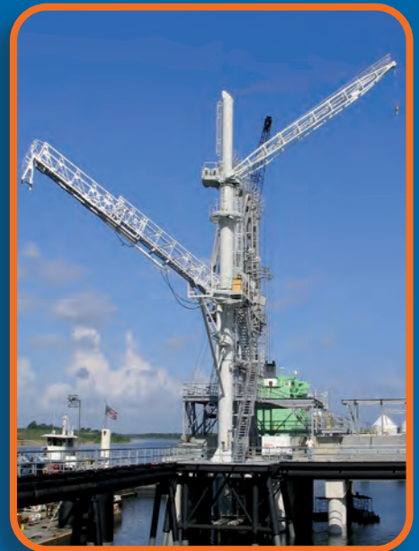
Column system in combination with hydraulic stores crane – Lake Charles, LA - USA.
