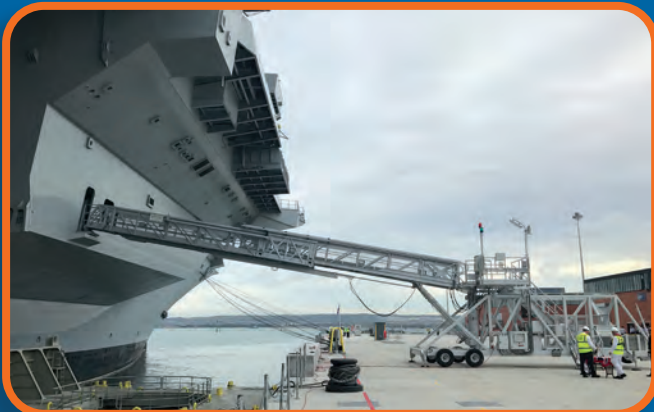
Hydraulically operated riding gangway system with telescopic ladder. Portsmouth - United Kingdom.
