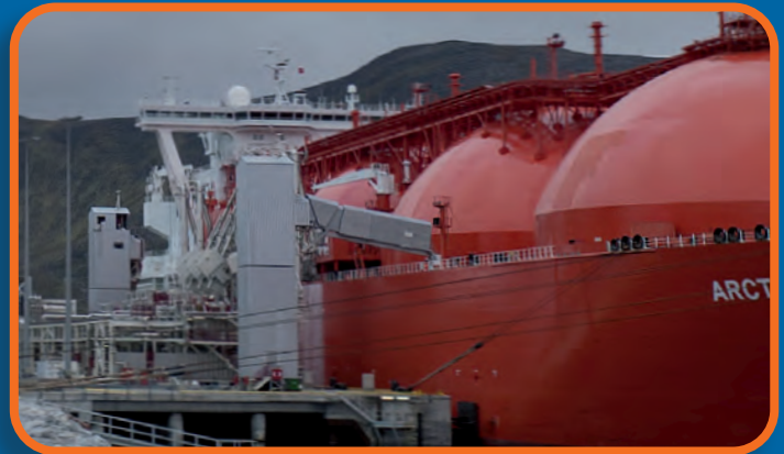
Covered gangway towers to withstand the extreme cold in Hammerfest - Norway.
